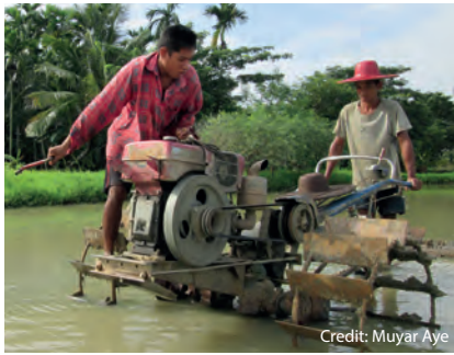
Paddy land preparation is mostly done through power tillers in Delta.
